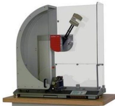
Gambar 6 mesin uji impak standar ASTM D6110 [11]
